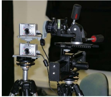
Fig. 1. Stereo bench setup. The 2 cameras are placed in vertical epipolar position
