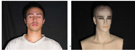
Fig. 3. Projection of a coloured grid on stereo images of test subjects for creating the reference disparity maps
