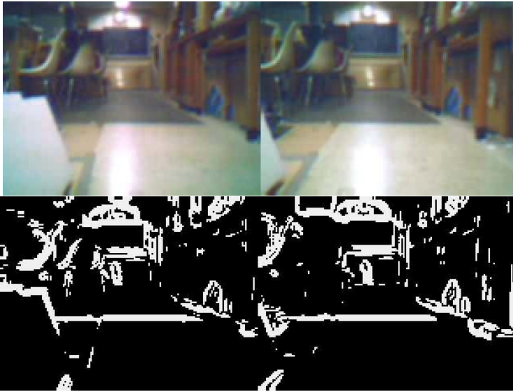
Fig. 9. The result of applying a Sobel edge detection to the blurred image
